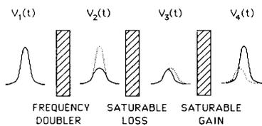
Fig. 1. Changes in the intracavity pulse envelope upon passage through major components of a passively mode-locked laser with an intracavity frequency doubler.
