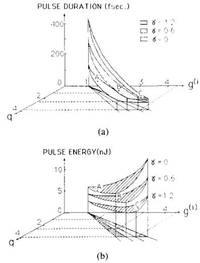
Fig. 3. Graphical representations of (a) intracavity pulse duration and (b) pulse energy at three different values of the second harmonic generation parameter  $\gamma$ . The points *A*, *B*, and *C* illustrate the simultaneous preservation of pulse duration and energy as  $\gamma$  is increased, and correspond to the equivalently labeled points in Fig. 2.
