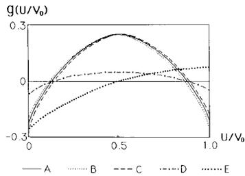
Fig. 4. Net gain parabolas showing gain versus normalized pulse energy from beginning ( $U/V_0 = 0$ ) to end ( $U/V_0 = 1$ ) of the pulse. Curves *A*, *B*, and *C* correspond to the points *A*, *B*, and *C* in Figs. 2 and 3, and show net loss before and after the pulse and net gain during the pulse, indicating mode-locking stability. Curve *D* depicts a stable condition of lower pulse energy and longer duration, while curve *E* depicts an unstable condition.
